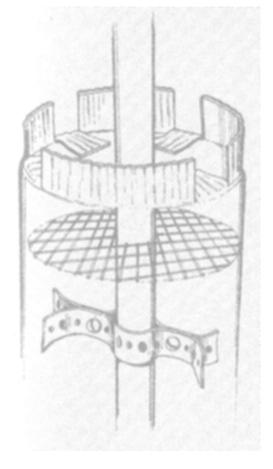
Make the baffle by cutting ½ inch hardware cloth into a 9 inch circle. Make a small hole in the center so that the circle will slip over the mounting pole (be sure to keep hardware cloth very close to pole and not leave any gaps (a one inch snake can get through a half inch hole).
